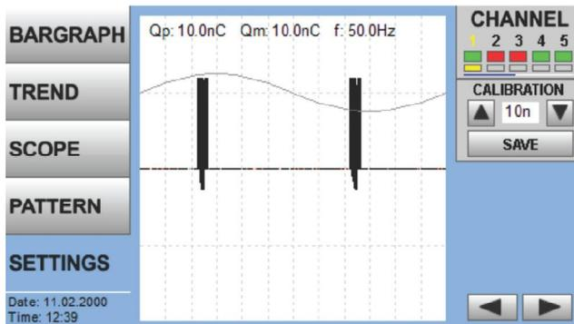
Fig. 8: Automatic pulse level detection
