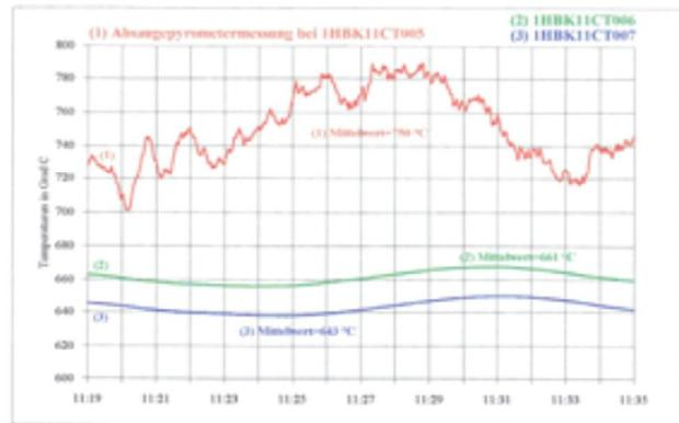
Fig. 1: Comparison of measurements made with thermocouples (green and blue traces) and a radiation free suction pyrometer (red trace) at the same position.
