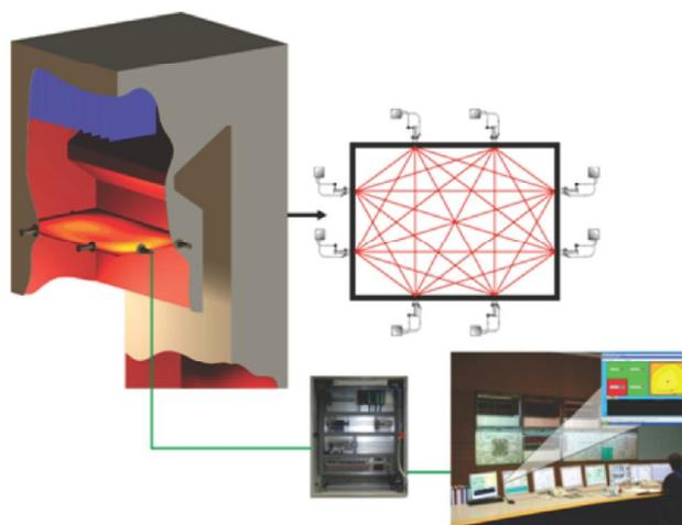
Fig. 8: Multiple paths arrangement at the furnace exit
