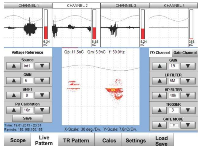
Fig. 11: Real Time Live phase resolved partial discharge Pattern
