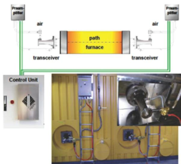
Fig. 7: Schematic representation of an acoustic temperature measuring system
