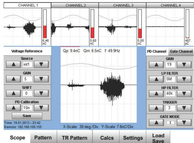
Fig. 10: Oscilloscope Scope View in Persistence Mode
