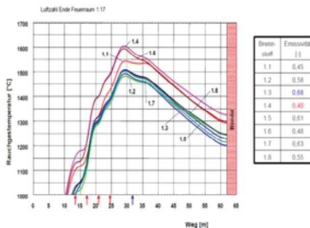
Fig. 4: Variation of FEGT for hard coal with different emissivity values  $\epsilon$  [1]
