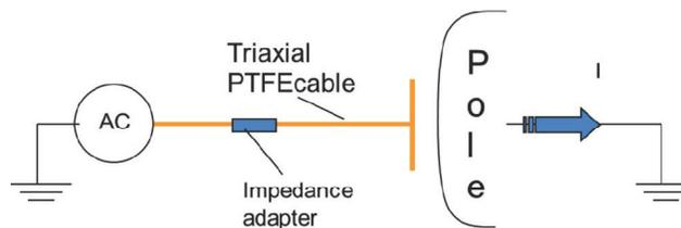
Fig. 5 : Airgap Transducer measuring principle
