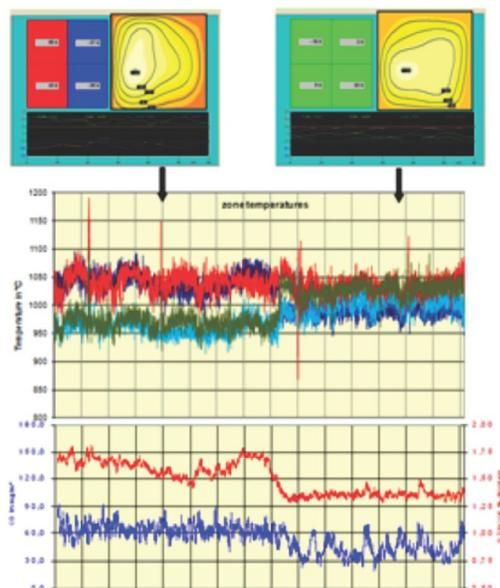
Fig. 12: Effects of temperature balancing on 4 zone temperatures above, O<sub>2</sub> (red) and CO (blue), 800 MW lignite
