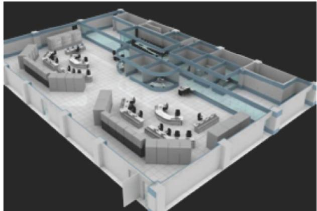
Fig 1: Typical MCR for 700 MWe NPP
