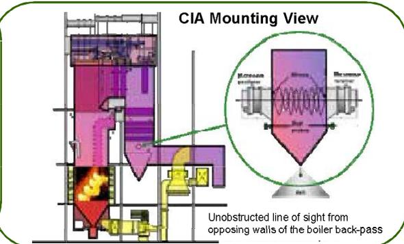
**Carbon in Ash offers Real time (24X7) Online monitoring of un-burnt carbon based on Non-Extractive methodology !**
