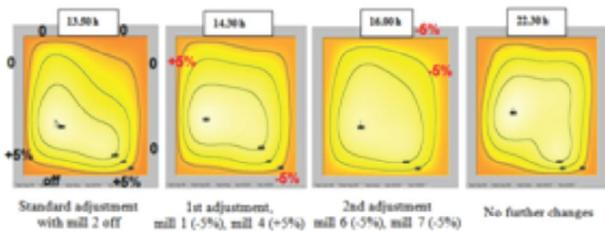
Fig. 11: Configuration of an acoustic system at the furnace exit of an 800 MW boiler. Below, typical temperature distributions made during balancing.
