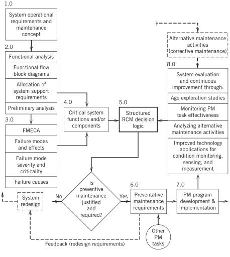
FIGURE 1: RELIABILITY-CENTERED MAINTENANCE ANALYSIS PROCESS. (Courtesy Blanchard and Blyler)
