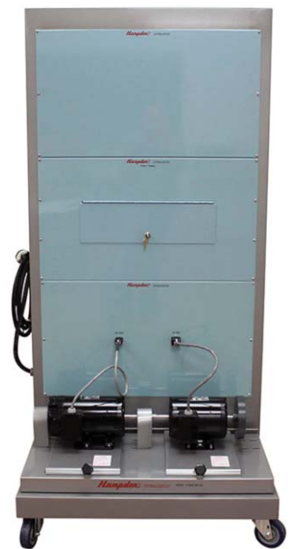
Rear view of the Hampden H-REM-ACDC-MC with standard DC Motor and AC Squirrel Cage Induction Motor
