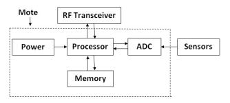
Figure 2. Block Diagram of Sensor Node
