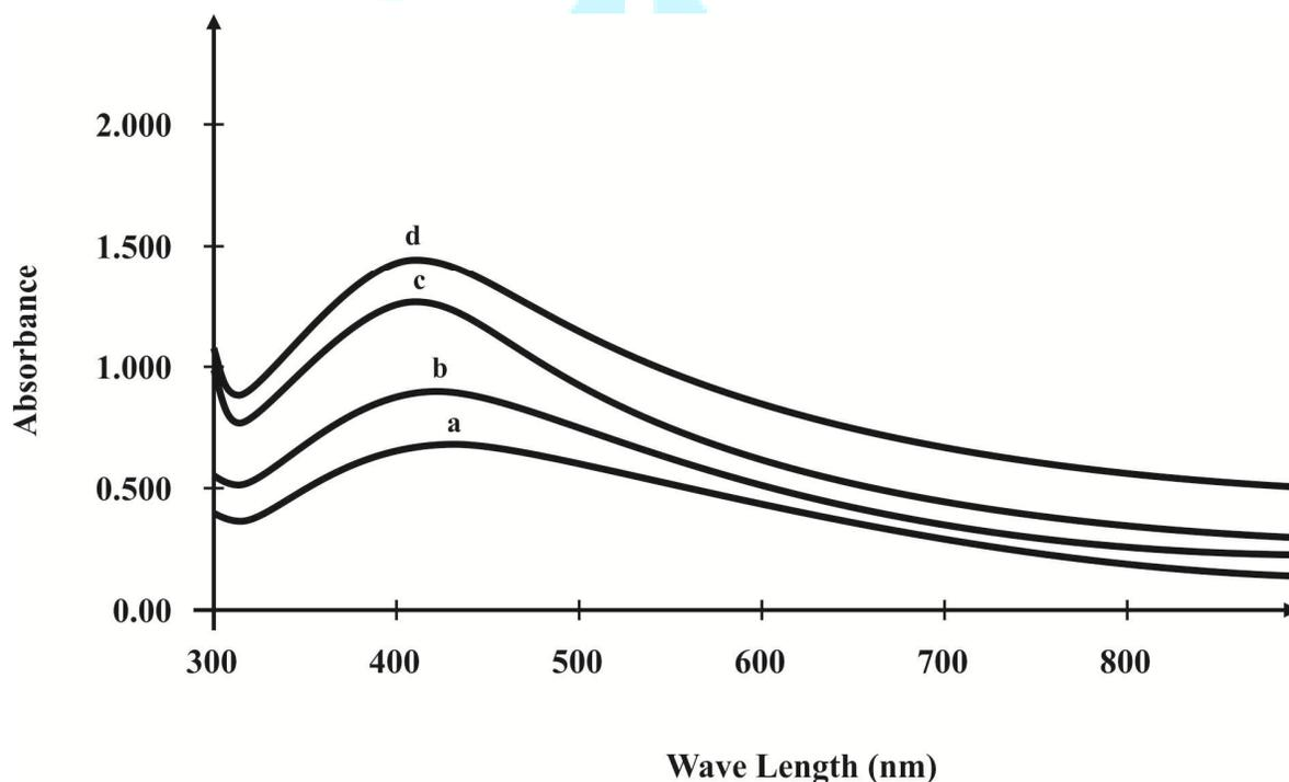
Fig. 1. UV-Visible spectrum of AgNPs (a) 420 nm for uncapped Ag (b) 416 nm for  $\alpha$ -CD (5 mM) capped Ag (c) 410 nm for  $\alpha$ -CD (10mM) capped Ag and (d) 408 nm for  $\alpha$ -CD (15 mM) capped Ag
