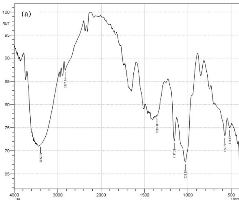
Fig. 3(a). FT-IR spectrum of  $\alpha$ -CD
