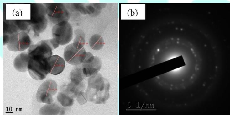
Fig. 4. TEM pictures of Spherical silver nanoparticles (a) 5 mM  $\alpha$ -CD capped, AgNPs (b) Selected area diffraction images of randomly selected AgNPs
