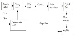
Fig.1: A block diagram of VLC
