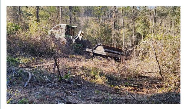
Above: **Roller Chopping**, AKA Drum Chopping, last fall in Stewart County GA on a Matre Forestry client tract, after a mid summer herbicide treatment and prior to longleaf planting by hand.
