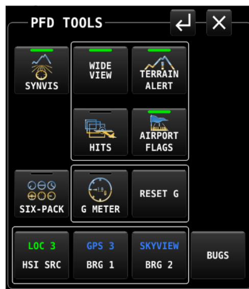
Figure 52 Bearing Pointer Selector in PFD TOOLS
