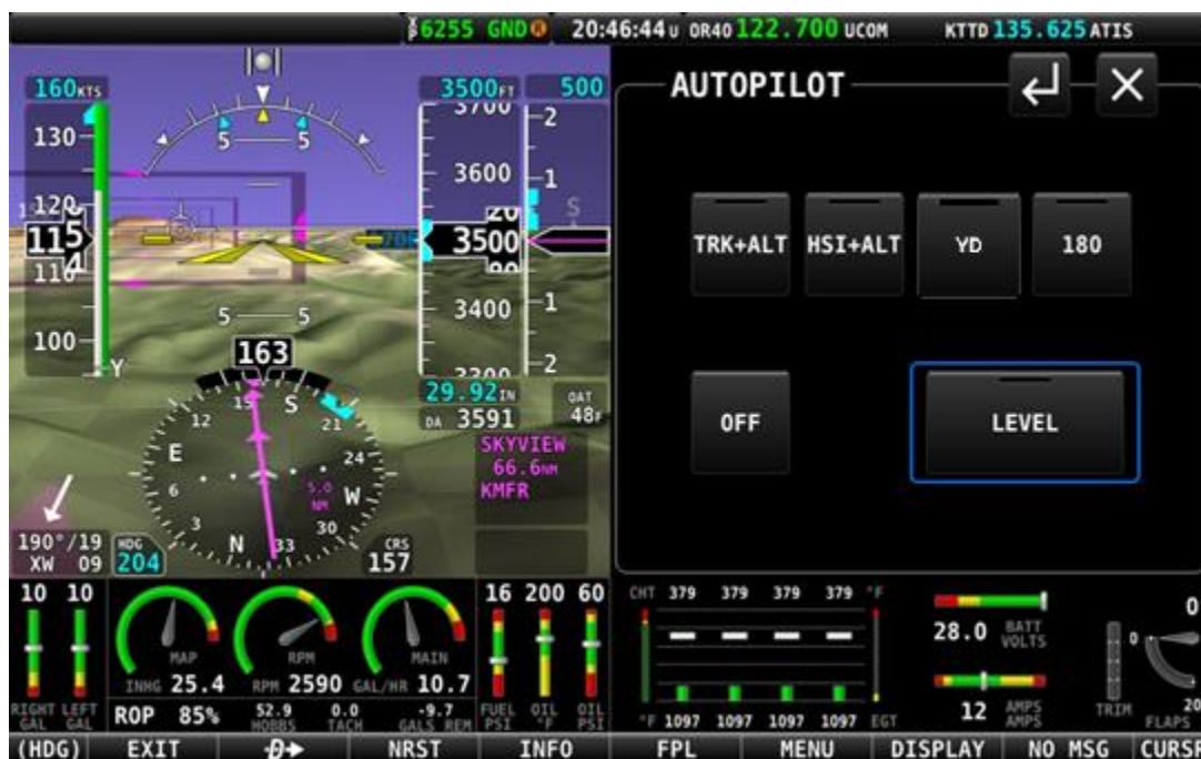
Figure 225 – AUTOPILOT Control page – Simplified Control Scheme
