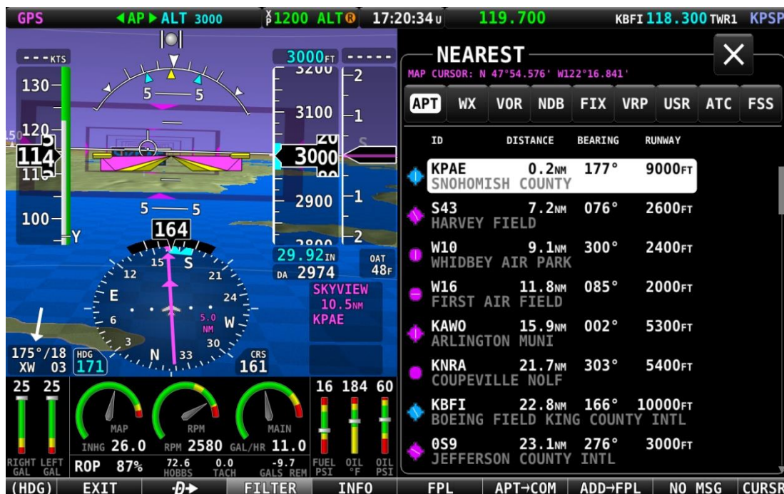
Figure 134 – Moving Map Nearest Window - FILTERED
