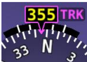
Figure 42 – GPS Track substitute for Magnetic Heading
