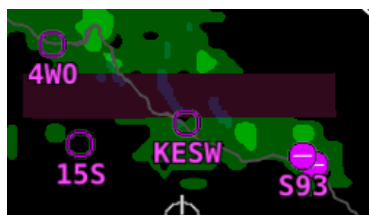
Figure 186 – Missing NEXAD Data Blocks
