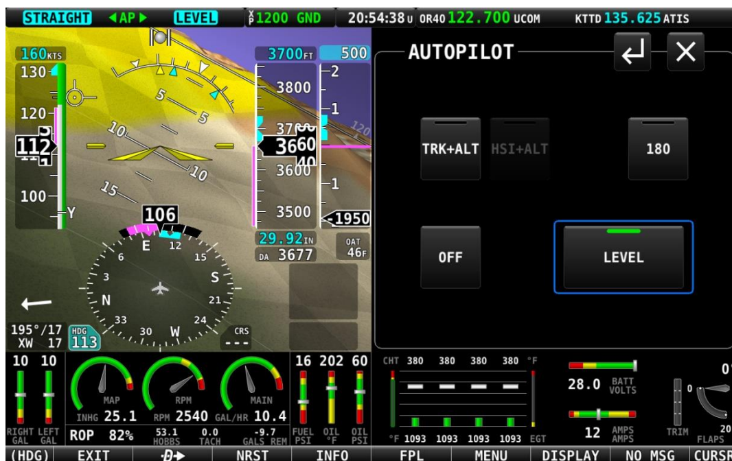
Figure 229 – LEVEL mode is engaged
