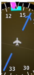
Figure 48 – HSI Bearing 1 Pointer
