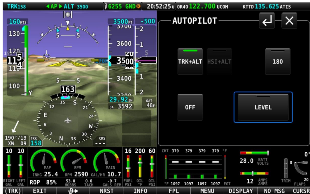
Figure 226 – TRK+ALT mode is engaged
