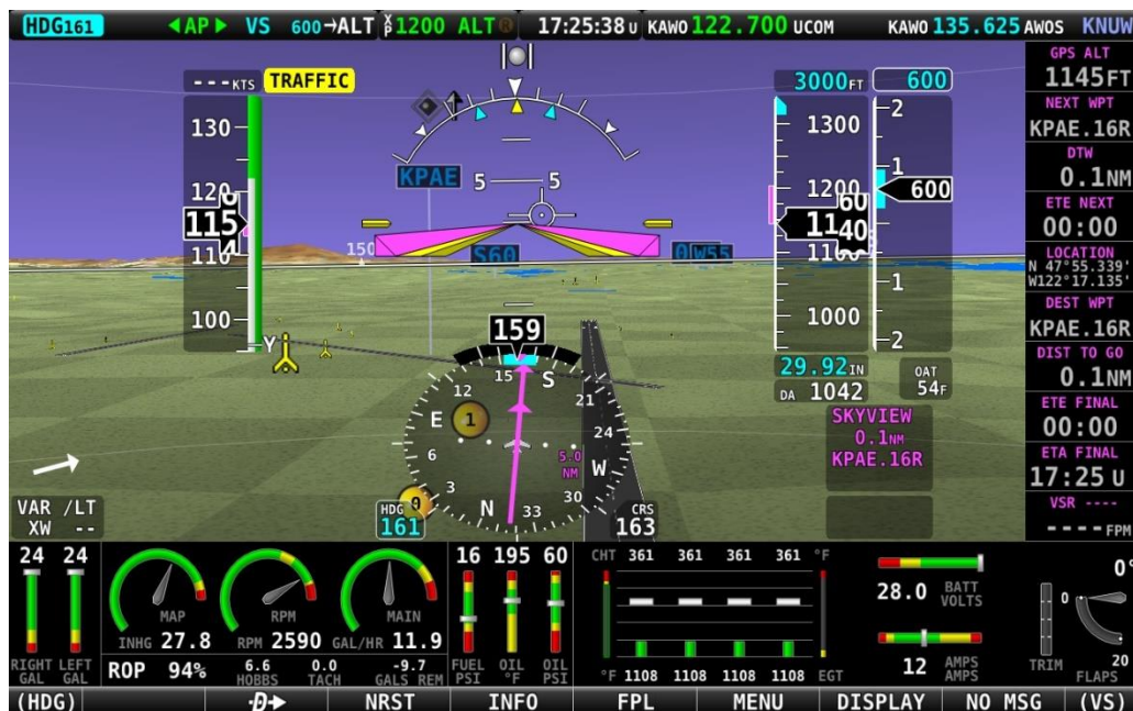
Figure 70 – SkyView HDX Synthetic Vision Traffic Alert
