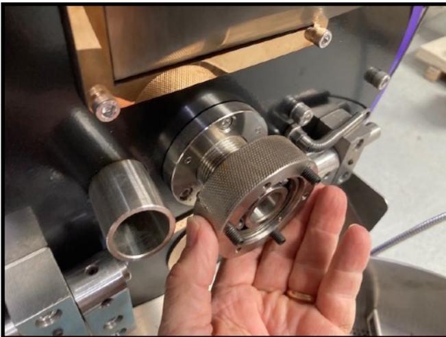
**11. IF NEEDED YOU MAY TAP BEARING FURTHER INTO HOLDER IF NOT FULLY INSERTED**
