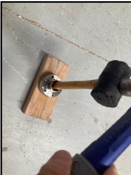
**6. SET HOLDER ON A BLOCK OF WOOD AND USING A WOOD HANDLE OR WOOD DOWEL ROD TO TAP OLD BEARING OUT OF HOLDER**
