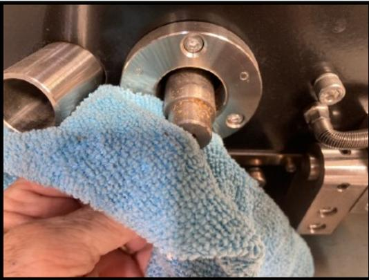
**8. CLEAN DRUM SHAFT OF DEBRIS. IF YOU LIKE YOU CAN PUT A THIN COATING OF GREASE ON SHAFT**
