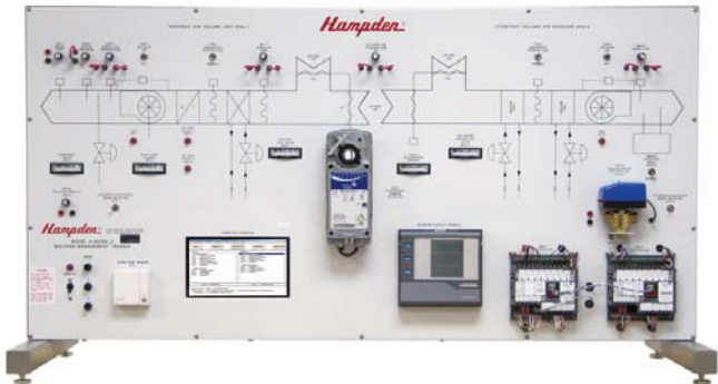
Hampden H-MZBM-J1 Multi-Zone Building Energy Management Trainer with industry standard JOHNSON CONTROLS
