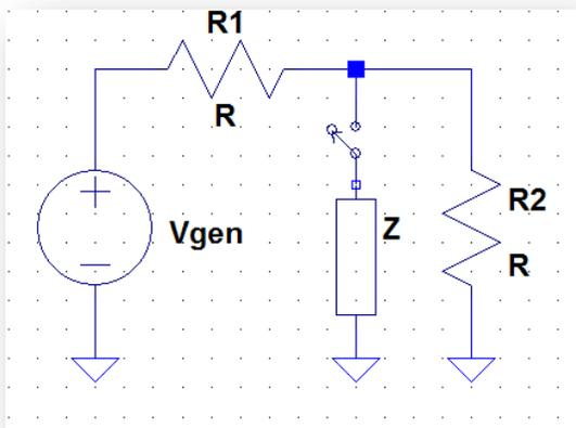
When Z is a resistance, the ratio of output voltage with Z connected to Z disconnected is easily calculated.
