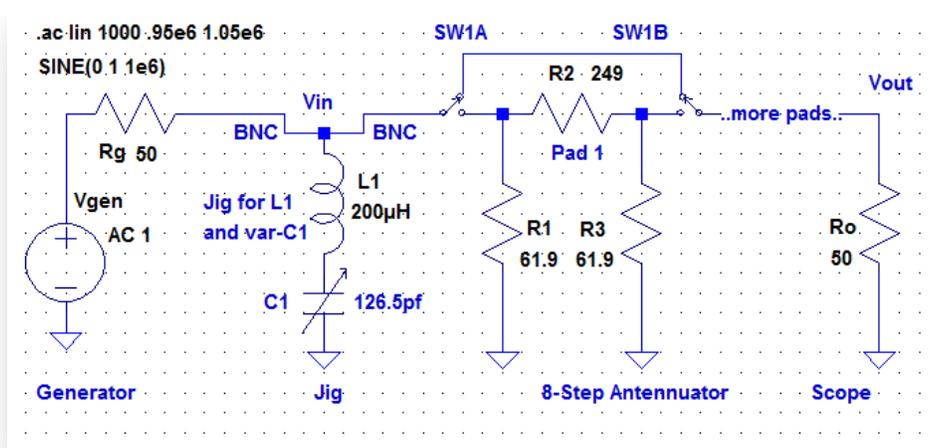
Figure 2: Simulation of Trap Q System
