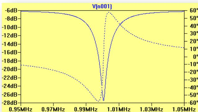
1. The generator is set for 1 volt at 1 MHz. The pad switches are pushed up to bypass the pads. With L1,C1 tuned much higher or lower than 1 MHz or with the them switched out of the circuit, the voltage at Vout will be 1/2, or -6 dB, as noted in the simulation output, Figure 2.
