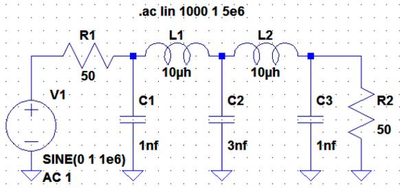
Figure 4B: Frequency Sweep of the Filter
