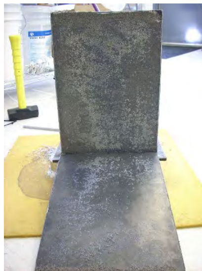
Figure 5. The mold with the finished shielding block, opened for testing
