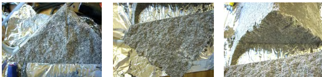
Figure 6. Faces of the shielding block after being broken open
