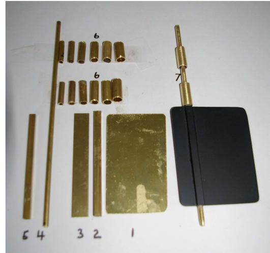
The rudder blade is made up from items 1, 2 and 3 shown. Items 1 and 3 are brass sheet, and item 2 is square section tube. They are soldered together in the same way that Garth and Steve made their open rudders.
