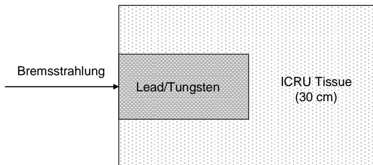
Figure 1. EGS4 simulation geometry of the APS safety shutters.
