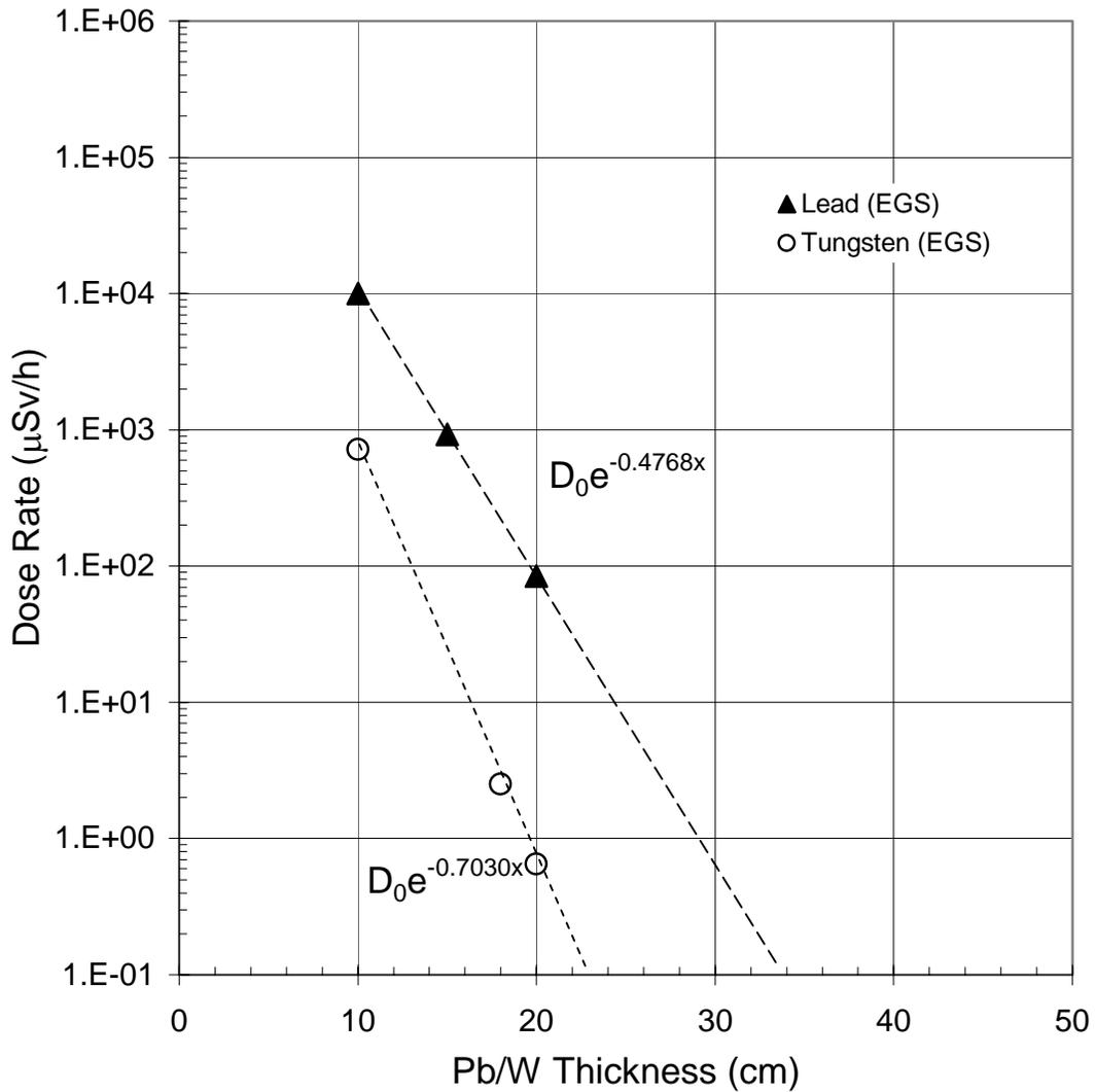
**Figure 4. Dose rates 30 cm downstream of the APS safety shutters (EGS4 calculation).**
