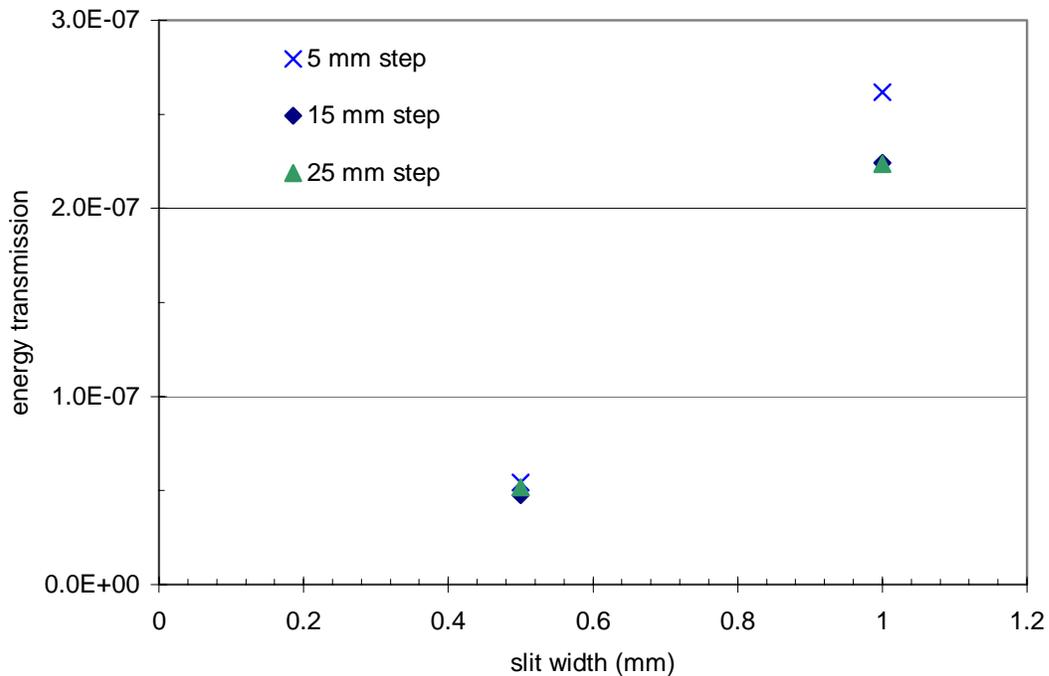
**Figure 11. Energy transmission vs. slit width for the APS tungsten bremsstrahlung shutters (photon beam normally incident at edge of opening in shutter). The same data are shown as in Figure 8 for energy transmissions in the range 0 to  $3 \cdot 10^{-7}$ .**
