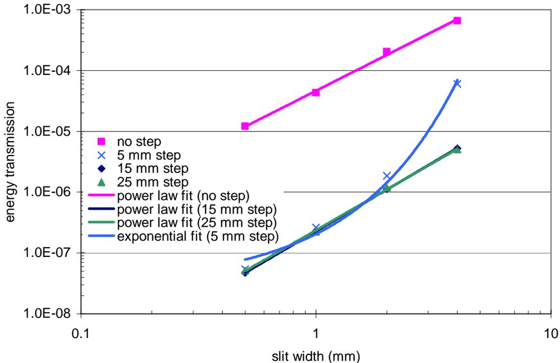
**Figure 7. Energy transmission vs. slit width for the APS tungsten bremsstrahlung shutters (photon beam normally incident at the edge of the opening in shutter).**
