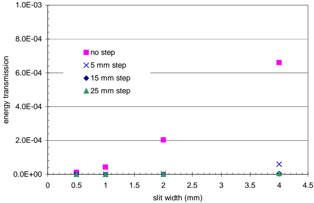
**Figure 8. Energy transmission vs. slit width for the APS tungsten bremsstrahlung shutters (photon beam normally incident at edge of opening in shutter). The same data are shown as in Figure 7, but with linear scales along each axis.**
