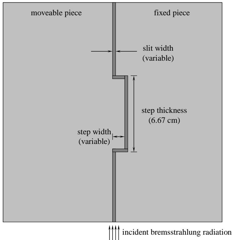
**Figure 2. Plan view of MCNPX geometry for APS safety shutters.**
