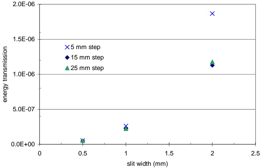
**Figure 10. Energy transmission vs. slit width for the APS tungsten bremsstrahlung shutters (photon beam normally incident at edge of opening in shutter). The same data are shown as in Figure 8 for energy transmissions in the range 0 to  $2 \cdot 10^{-6}$ .**
