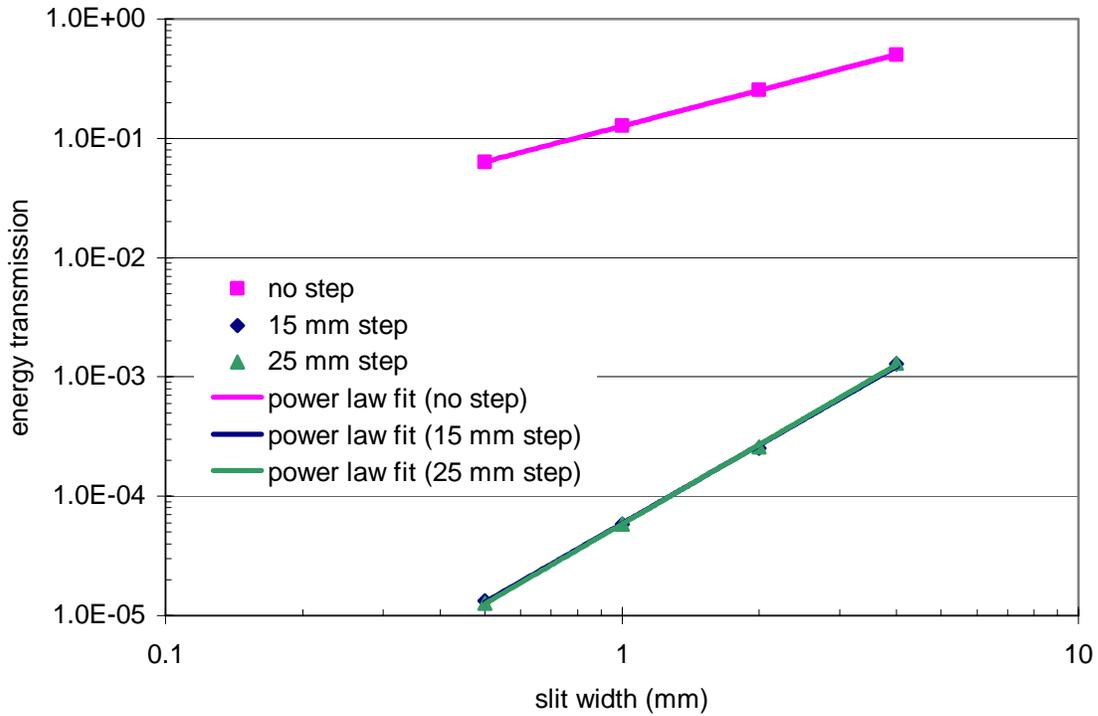
Figure 5. Energy transmission vs. slit width for the APS tungsten bremsstrahlung shutters (photon beam normally incident on opening in shutter).
