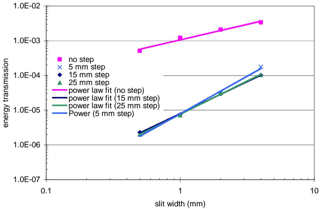
Figure 6. Energy transmission vs. slit width for the APS tungsten bremsstrahlung shutters (photon beam obliquely incident on opening in shutter).
