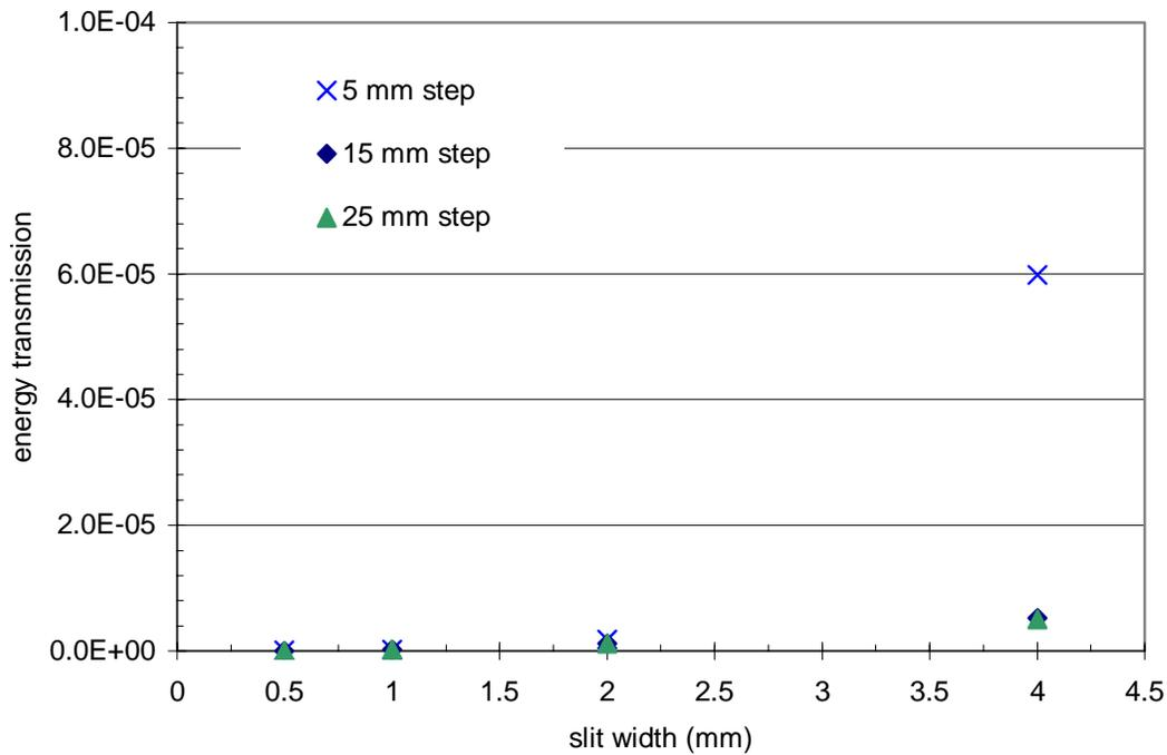
**Figure 9. Energy transmission vs. slit width for the APS tungsten bremsstrahlung shutters (photon beam normally incident at edge of opening in shutter). The same data are shown as in Figure 8 for energy transmissions in the range 0 to  $10^{-4}$ .**
