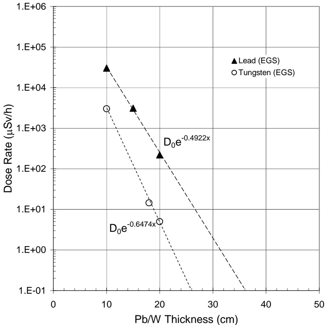
**Figure 3. Contact dose rates at the downstream surface of the APS safety shutters (EGS4 simulation).**
