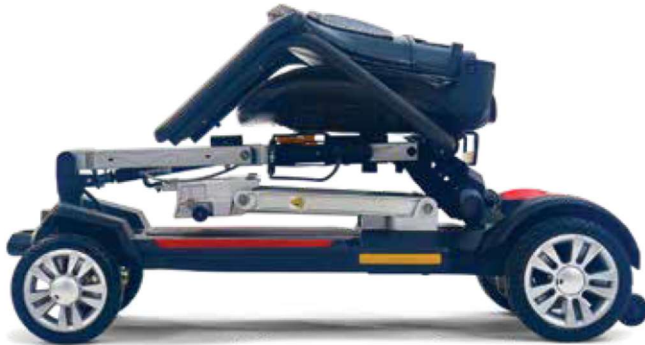
Tiller & self-locking seat frame fold for a compact profile
