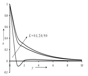
Fig.3: The dimensionless velocity verses various values of K when Sc=0.22, Kc=0.2, R=0.3, Pr=2.0, F=3.0, M=2.0, Gr=1.0, Gc=0.5 and Ec=0.01
