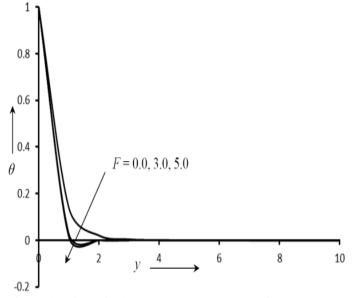
Fig.5: The dimensionless temperature verses various values of *F* when Sc=0.22, =0.2, R=0.3, Pr=2.0, M=2.0, K=2.0, =1.0, =0.5 and Ec=0.01.
