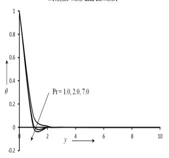
Fig.4 :- The dimensionless temperature verses various values of Pr when Sc=0.22, =0.2, R=0.3, F=3.0, M=2.0, K=2.0, =1.0, =0.5 and Ec=0.01
