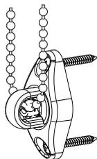
4. Lower and raise the shades to confirm smooth operation including proper setting of the stops. Confirm control chains are routed properly. Check before and after installing tension devices.
