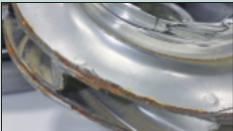
SAND-DAMAGED SUBMERSIBLE PUMP IMPELLER
