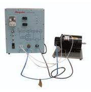
The Model H-ACVD-100 AC Vector Drive Trainer System provides students with hands-on experience with advanced motor controls. It is available in two configurations; as a stand-alone trainer and as an adjunct trainer to the Hampden Series 100 Rotating Machine System. Either system is designed for bench top mounting or may be used with the optional Model HMT-4 Mobile Table.
