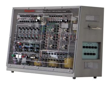
The **Model H-R-SCR-2** Power Electronics System provides students the opportunity to investigate diode rectifier circuits and AC & DC controlled power circuits utilizing silicon controlled rectifiers (thyristors) with resistance, capacitance, and unijunction transistor (UJT) triggering.
