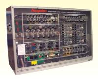
The **Model H-R-SCR-1A** provides students with the opportunity to investigate diode rectifier circuits and AC and DC controlled power circuits and unijunction transistor (UJT) triggering.
