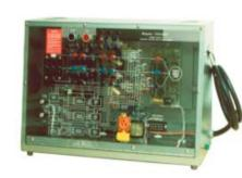
The Model H-RVS-2A 3Ø AC Reduced Voltage solid-state Starter provides students with experience in connecting, testing, and operating a commercially-available solid state reduced voltage starter for three-phase induction motors
