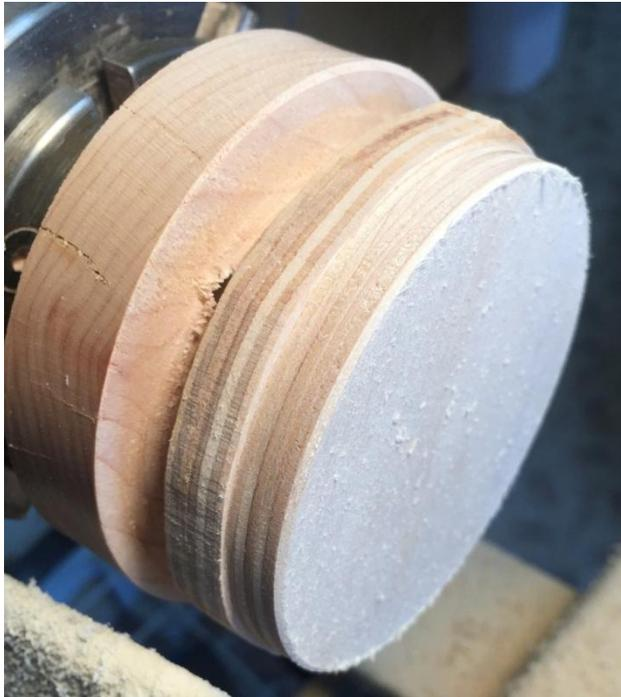
Here's a picture of the rotary disk being rounded while mounted on the screw chuck. Note the lack of a hole in the front side. Once I got half the disk rounded true, I dismantled the disk from the screw chuck and mounted it in grooved jaws to cut the back-side bevel.
