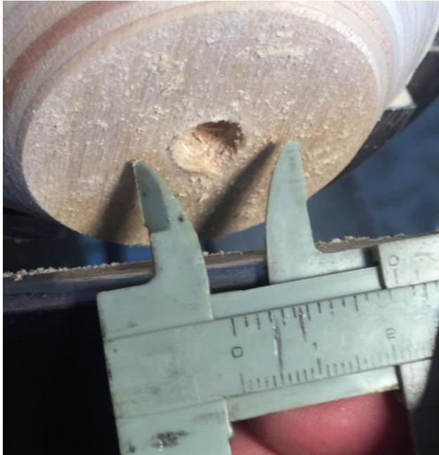
Next, you transfer the 22 mm diameter to the backside of the rotary sanding disk. The cheap plastic calipers won't scribe the plywood, but a sharp awl did the trick just fine, once I knew where to hold it.
