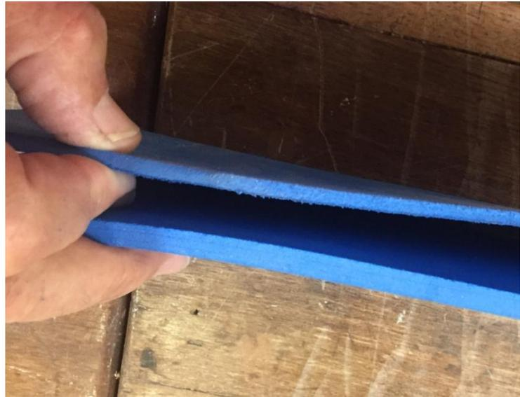
The different thickness of the two pieces is not an accident. One side of the floor pad is smooth, but the other side is pebble grained. I resaw twice to remove the pebble grain. Bet you didn't know and wouldn't believe that you could resaw a flexible foam pad so thinly. I approached the project with great caution, and my first bit of cutting was done with fingers well back, and a very slow feed.
