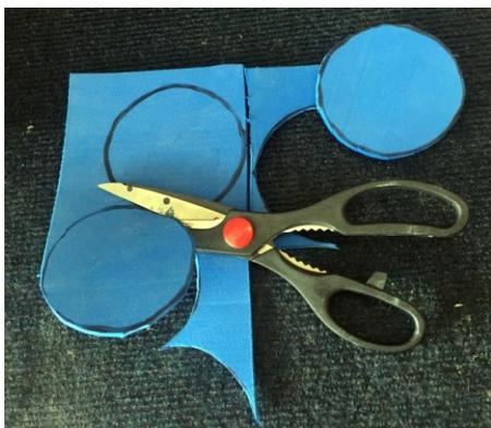
Next, use one of your wooden rotary disks as an outline, and draw circles on the foam. Then cut the foam out with a pair of shop scissors from Harbor Freight. The foam cuts very easily, but it does dull the scissors rather quickly, so a free pair of scissors from Harbor Freight is just the ticket for this task.
