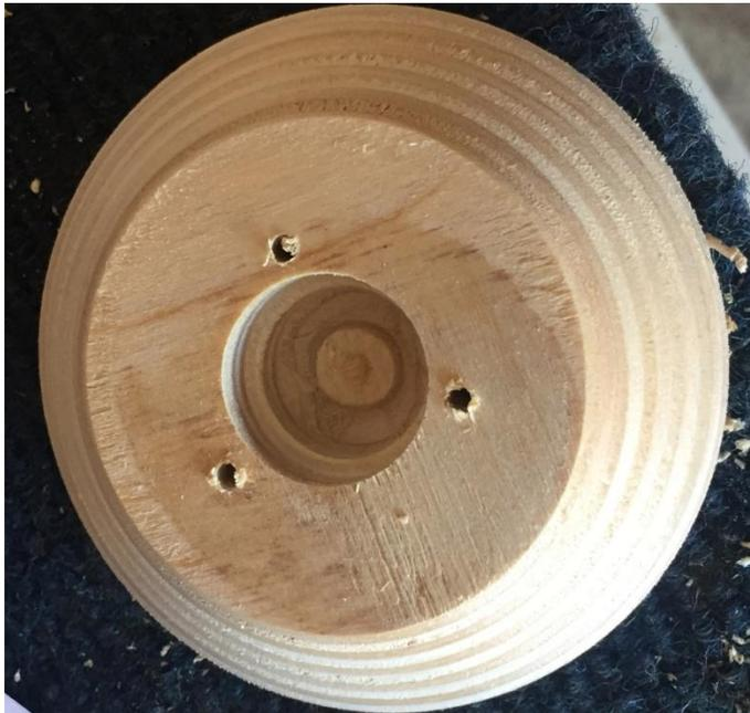
Once the bearing spins freely, remove it, and drill three pilot holes for the retainer screws that will hold the bearing and bolt head in place. You want the head of the retainer screws to reach out over the outer bearing race, but not much further, lest you compress the sealed bearing cover.
