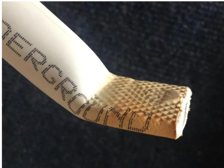
Now, repeat the heating, flattening, and bending of the other end of the conduit. Try, for aesthetic reasons, to keep the two ends bent on the same axis. It doesn't matter a bit if they are not quite on the same axis, but it sure looks better if they are. Do as I say, not as I did on my first one!
