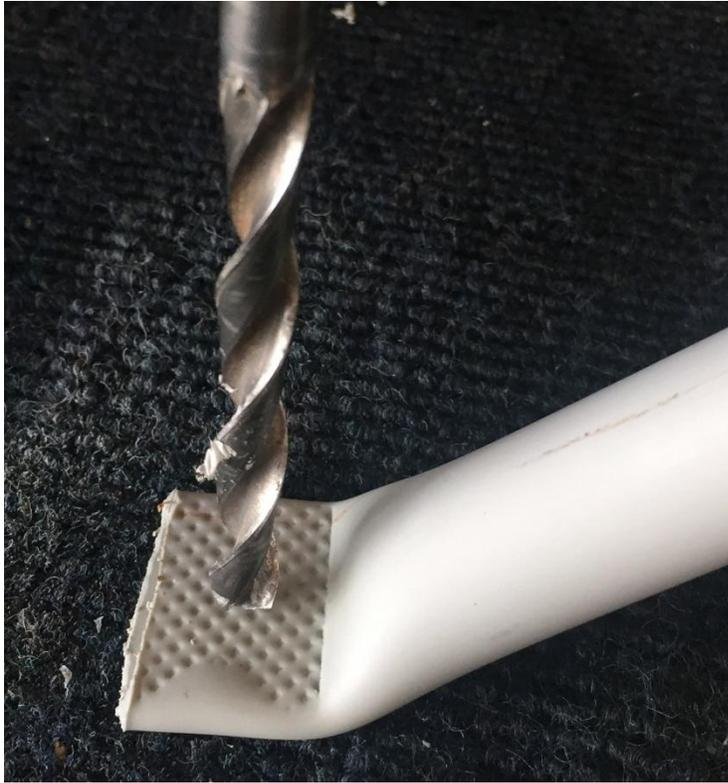
Drill a 5/16-inch hole in each end of the conduit.
