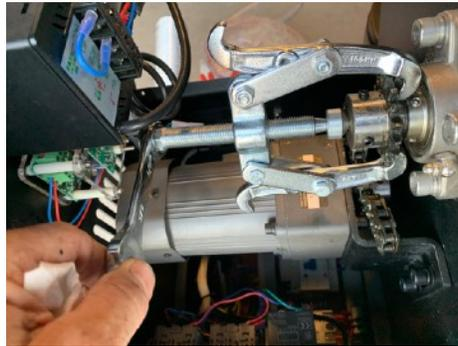
Once Chain Sprocket is removed you will have access to the Back Bearing:
