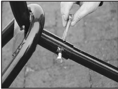
Step 5 Put in Bolt to Hold Main Frame to Draw Bar.
