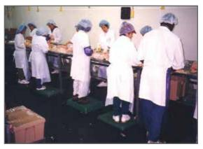
and grating rubber feet, any size work mat can be created. The feet raise the grating 1/2" above the ground and the open mesh allows chips and fluids to fall below the standing surface providing a safe, clean working area. Should your operations require more complex work stations, Fibergrate's turnkey approach includes design, fabrication and installation services for everything from a simple portable station to larger fixed platforms with railings and stairways.
