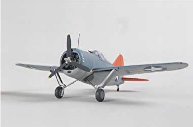
Prior to assembling the fuselage, I used a razor saw to remove the engine cowling from the two fuselage halves. I finished up the kit's cockpit and glued the fuselage together, then used super glue to attach the resin extension to the front of the fuselage. After sanding and filling the joint, I turned to the now separate cowling.
