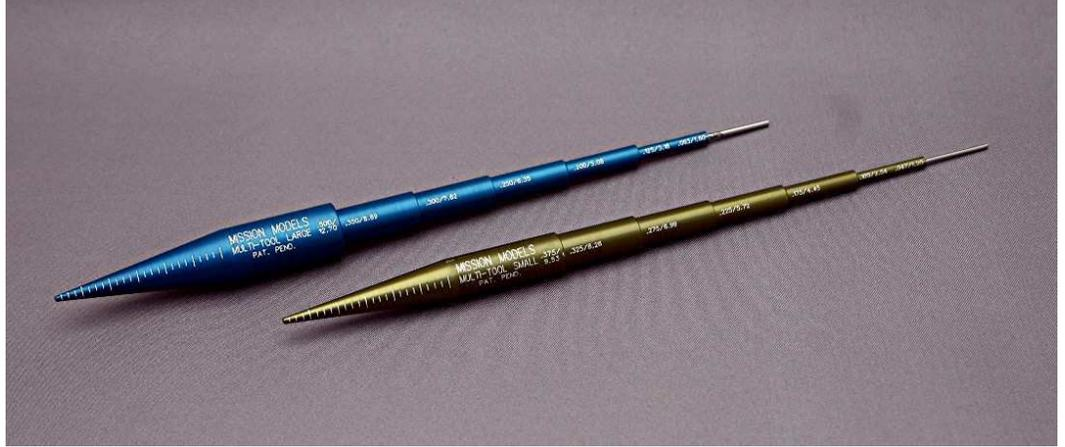
I am working on Academy's M-10, and had a few PE parts from Eduard's detail set that needed bending, particularly the light guards and shell racks. I didn't bother to heat the parts up beforehand, since they were rather small and thin. I trimmed them off the fret, positioned on the tool and gently pressed them into the desired curve. And, well "wow", it worked. Surprise.
