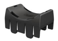
**Polymer Cable Saddles** are made from injection molded glass-filled polymer resin to create a strong, non-conductive cable saddle for use with underground cable support arms in vaults and manholes. The fiber-reinforced polymer saddles are non-corrosive for long-term durability. Emits no harmful smoke. Snaps onto the bracket arm and will not fall off. Easily secures the cable tightly to the saddle using one cable tie that travels under the saddle through opposing holes and a channel.
