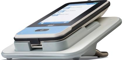
The Novus can handle a heavy test workload. A fully charged Novus will last for approximately 50 ABR screens and 150 OAE screens depending on test times. The Novus alllows for testing when in the charging cradle for times when the battery is low, ensuring no missed screenings.
