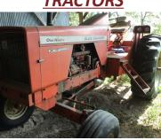
Allis Chalmer 190 XT Series III tractor, w/4 hydraulic outlets
