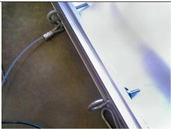
The tests consisted of two 36" pieces of different extrusions (TS32 & TS44) on which a 36" x 72" piece of 13 Oz. vinyl was fixed on each facing channels using a PVC locking strip.
