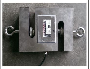
Here is the sensor measuring the applied force also called "Sensor Cell".
