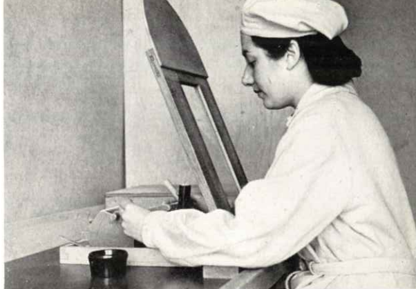
Filling Igniters ; screen protects worker's face.
