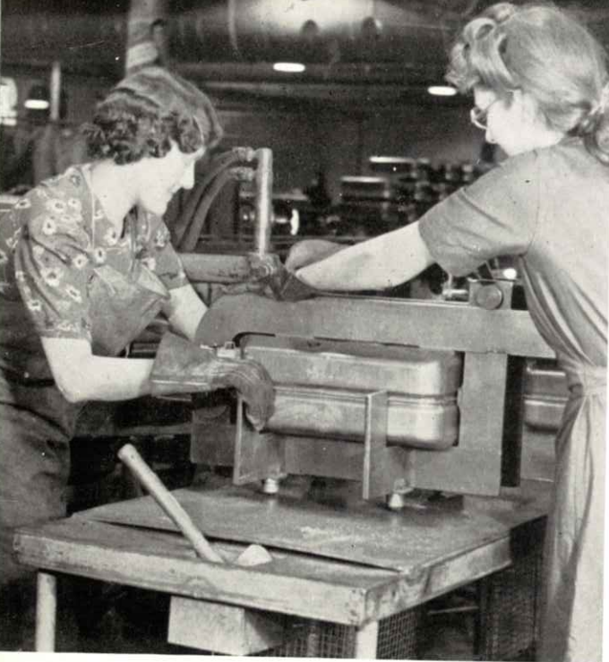
Spot-welding the two halves of a Ferrican before seam-welding.
