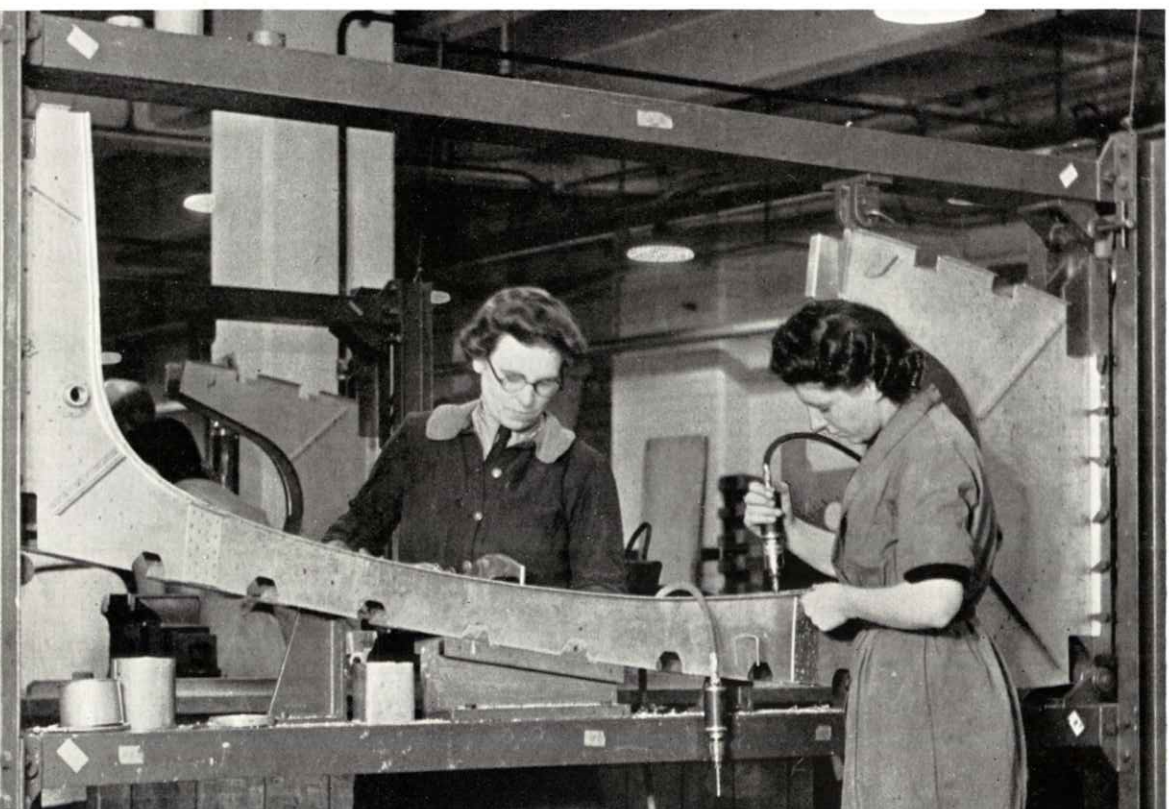
Drilling and riveting skins to large tank ribs.
