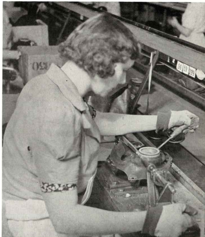
Screwing-up clip of eyepiece.
