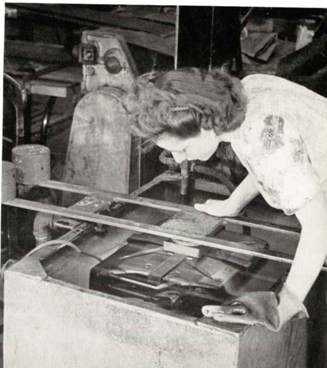
(Left.) Welding on the handle. (Right.) Testing for leaks by air pressure.
