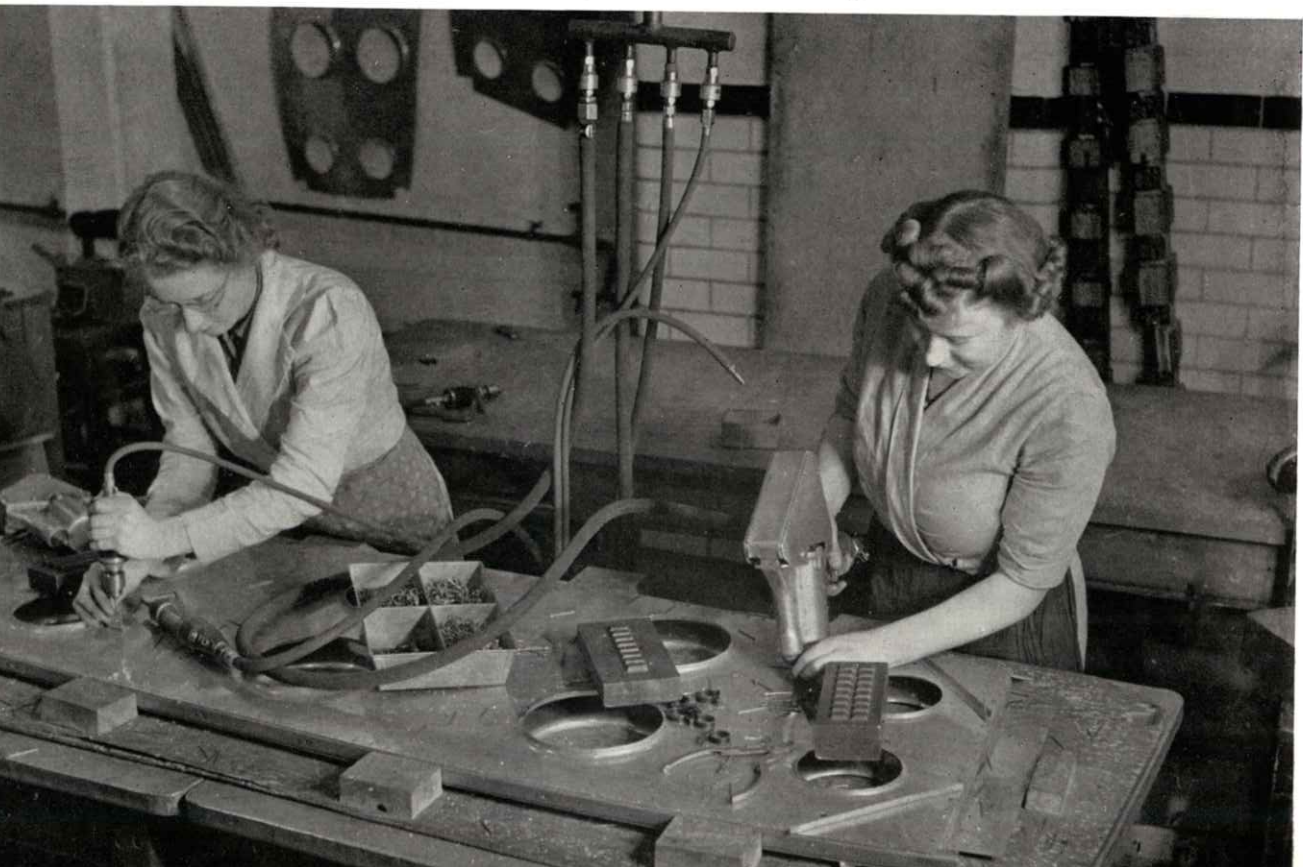
Lancaster Wing Rib. Riveting boom on to stiffener.
