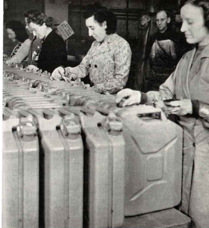
(Left.) Painted cans passing through an infra-red drying oven. Those intended for desert use were sand-coloured and others dark green. (Right.) Government inspection of completed containers.
