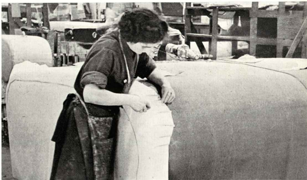
Covering a Lancaster tank with rubberized fabric: shaping the end.
