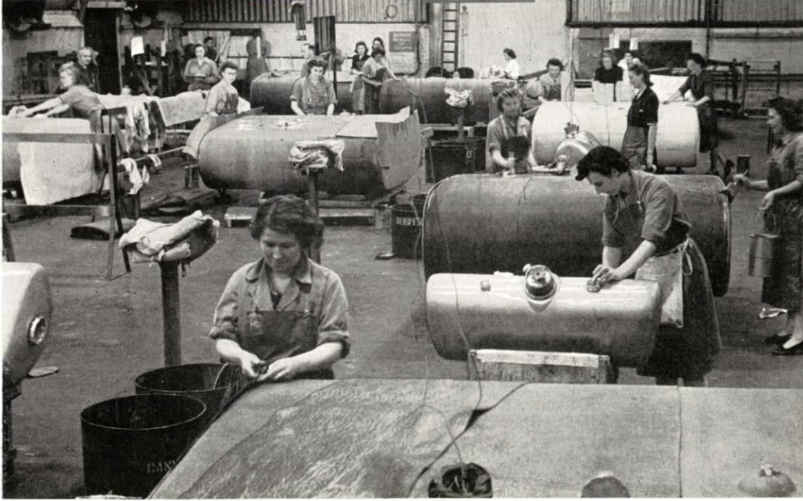
General view of Covering Room, showing Lancaster main tanks and Lancaster inboard oil tanks.
