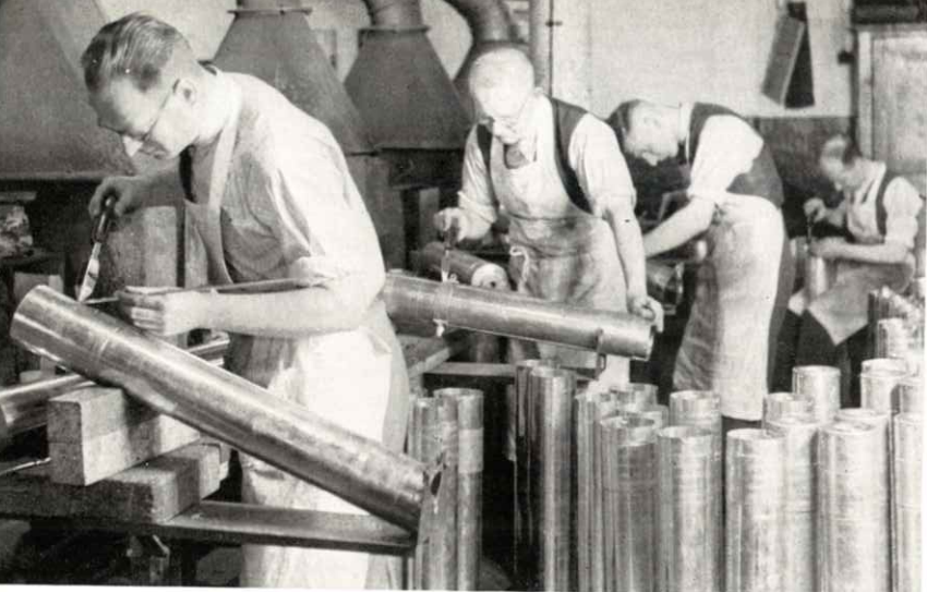
(Left.) Soldering vanes to Parachute Flares. (Right.) Testing bodies of Parachute Flares for leaks. This Mould-maker's job was one of the first that Bournville Utilities undertook.
