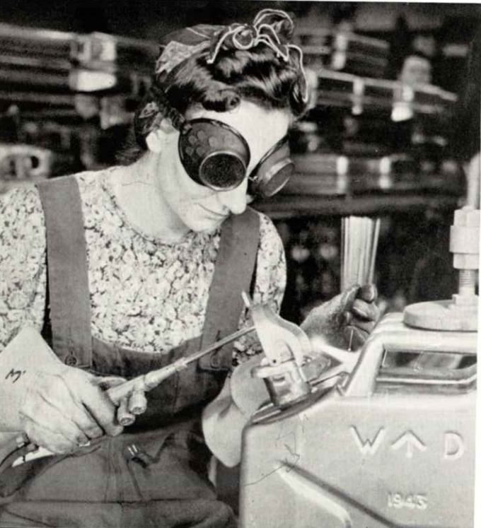
(Left.) Welding on the handle. (Right.) Testing for leaks by air pressure.
