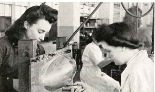
(Below) Gun-doors for Spitfires. The girl on the left is riveting while her companion holds the "dolly."
