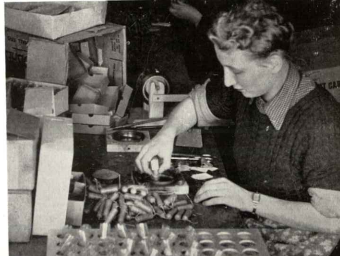
(Left.) Bomb Sight Brackets for Lancaster. (Right.) Sealing ends of cellulose tubes (Battersea Factory).
