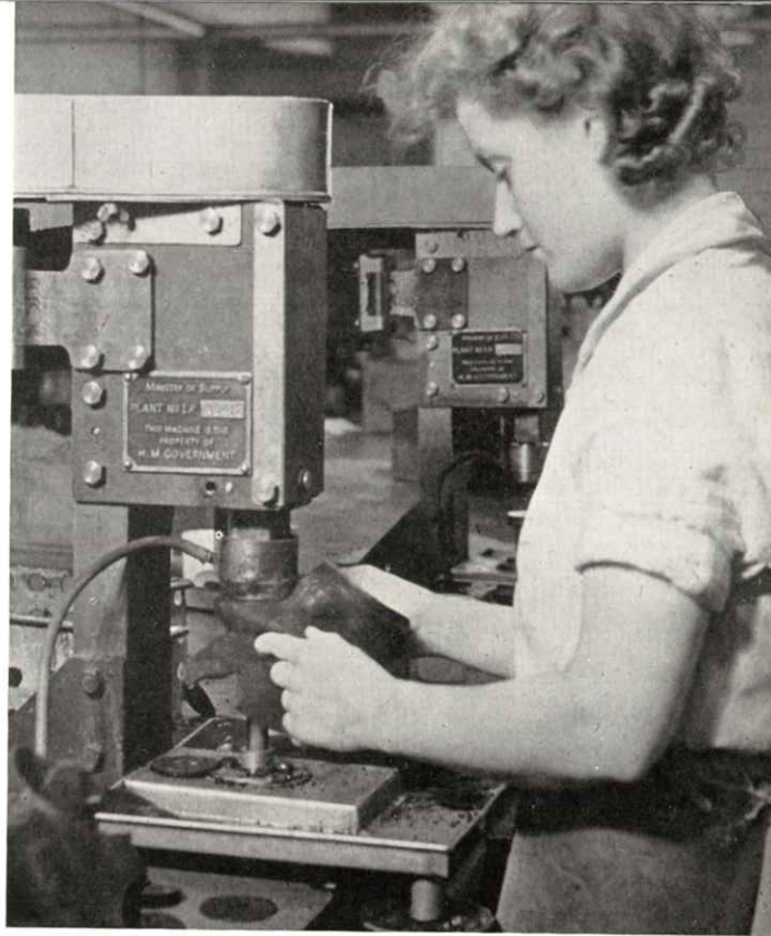
Cutting out 'flash' for eyepiece.
