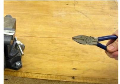
Be careful if you are trying to pull hard on a thick wire. Brace yourself in case the wire breaks or pulls out of the pliers.
