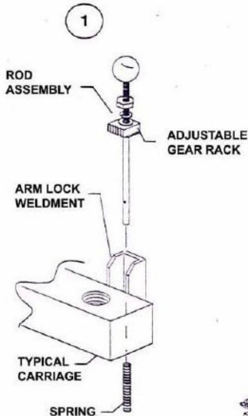
INSTALL COTTER PIN AS SHOWN TO ENSURE SPRING STAYS INPLACE.
