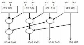
Fig.4:Schematic diagram of 4-bit Kogge-Stone Adder
