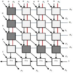
*Fig.2: Block diagram of 4 bit Baugh -Wooley multiplier B. Vedic Multiplier*
