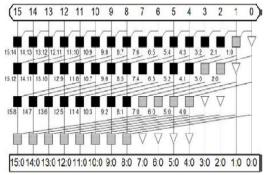
Fig.5: Schematic diagram of 4-bit Kogge-Stone Adder.
