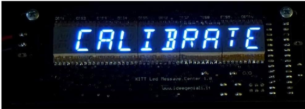
Display dimensions: 13x96mm; Board dimensions: 53x134mm
