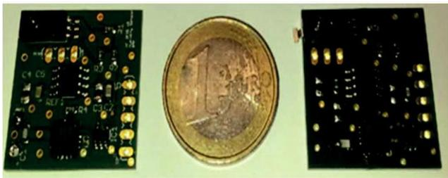
Figure (a) RFID sensor system (UHF left, HF right)
