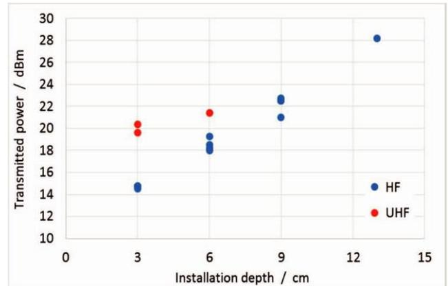
Figure (f) Comparison between the results of HF and UHF measurements.
