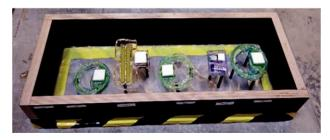
Figure (c) Test specimen with RFID systems before filling with concrete.
