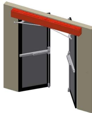
OUT/PUSH (doors swing away from Operators)
