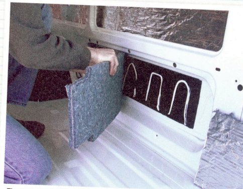
Figure 9. Application of Cascade Audio's Acoustical Cotton Composite using heavy-duty construction adhesive (ICI Paints' Liquid Nails PN LN-903) was used to bond the Acoustical Cotton to the VMAX.
