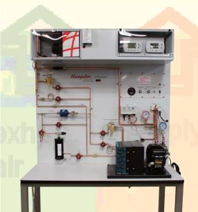
The Hampden Model H-RST-8 Heat Pump Trainer provides students with an introduction to the principal components of heat pump systems.
