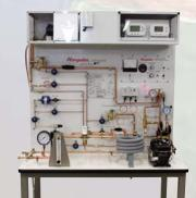
The Hampden Model H-RST-12 Heat Pump Trainer with water cooled condenser provides the student with an introduction to the principle components of heat pump systems.
