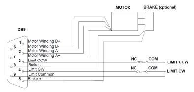
ADC uses a standard male DB-9 Connector for both the motor and limit switches.
