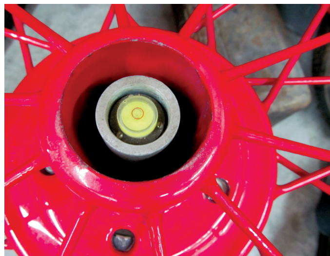
Once the weights are placed in the correct spot(s), the wheel comes in balance, centering the bubble in the dot. Mark the weight locations with ink marker on the inside of the rim. Placing the weights in this location will hide them, but keeps the balance just the same.
