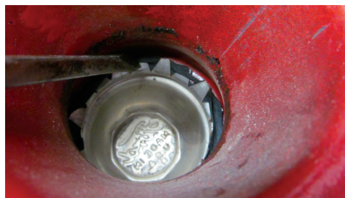
A tip for loose or rattling hub caps, as the thin tabs won't hold at times: Use a single layer of friction tape. Folding the thin tabs into the friction tape keeps the cap snugly tight!
