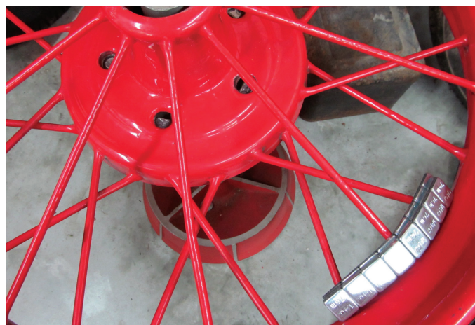
Notice strips of weights layered on the outer rim. Position strips for adjusting the location around the rim, separating segments of weights as needed. Sometimes balance is attained when segments are placed apart from one another.
