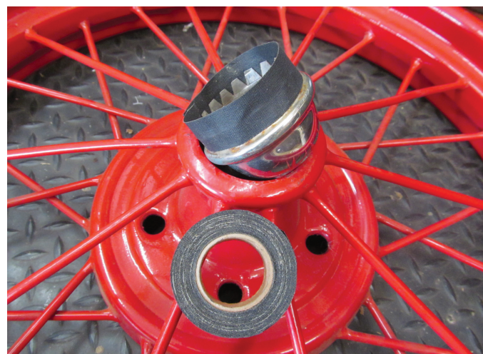
Notice strips of weights layered on the outer rim. Position strips for adjusting the location around the rim, separating segments of weights as needed. Sometimes balance is attained when segments are placed apart from one another.
