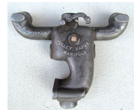
Photo of Vapor Manifold intake. Not pictured is the special exhaust manifold, with a central port connection, provided by Holley.
