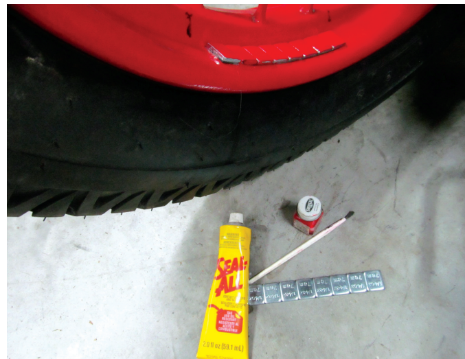
Adhere the weights to the inside of the wheel rim, using the ink marks as your guide. The 'sticky' of the adhesive weights was poor on the powder-coat finish on these particular wheels, so I applied a bead of contact cement (Seal All® or similar) to secure the weights in place. A coat of hobby shop enamel paint will mask the shiny metal weights.
