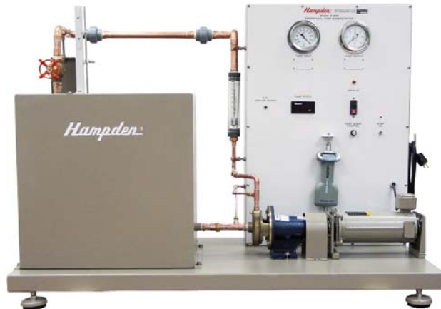
MODEL H-6981 Centrifugal Pump Test Demonstrator Dimensions: 40-3/4"H x 58-3/4"W x 28"D - Shipping Weight: 575 lbs.
