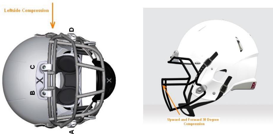
Figure 3a and 3b – Compression testing sites on the device and facemask
