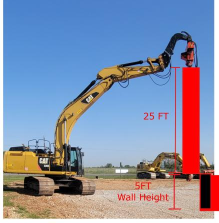
Sheet piling has interlocks. You must consider your sheet piling wall height, in order to determine the maximum length of sheets that you can drive with the gooseneck.
