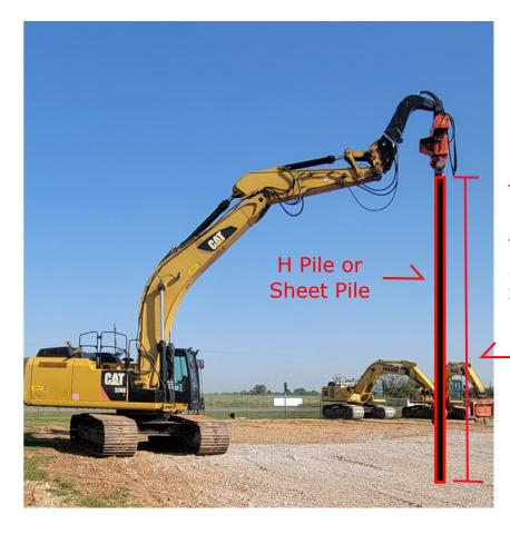
The Gooseneck Extension allows for lifting up to 30ft H piles or Sheet piles
