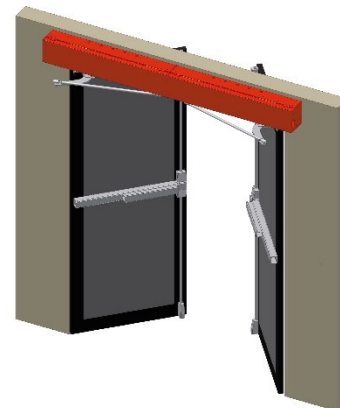
OUT/PUSH (doors swing away from Operators)
