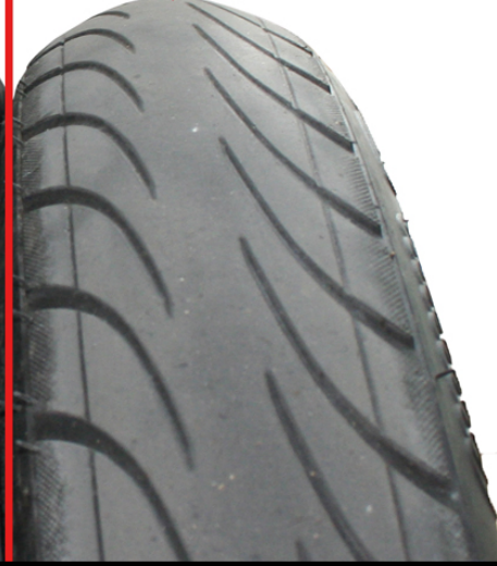
x2 TIRE THAT REQUIRES REPLACING
