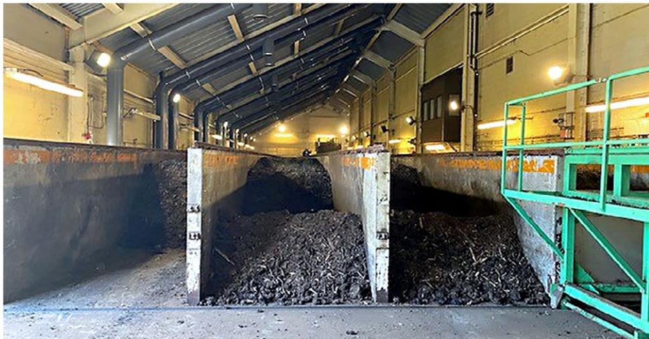
**The Town of Bennington, Vermont built an IPS agitated bay facility in 1992 at its wastewater treatment plant (WWTP) to compost biosolids with yard trimmings. The 4-bay Bennington Compost Facility utilizes equipment supplied by BDP Industries.**
