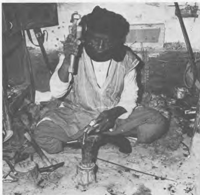
6-225 GOULIMENE, SOUTHERN MOROCCO. Jeweler forge hammering a small silver ingot on an anvil anchored in the earthen floor in preparation for use in forming a forged wire ornament. Photo: Oppi
