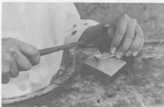
Figure 5.46 Hammering a workpiece with the peen of a hammer on the bench block.
