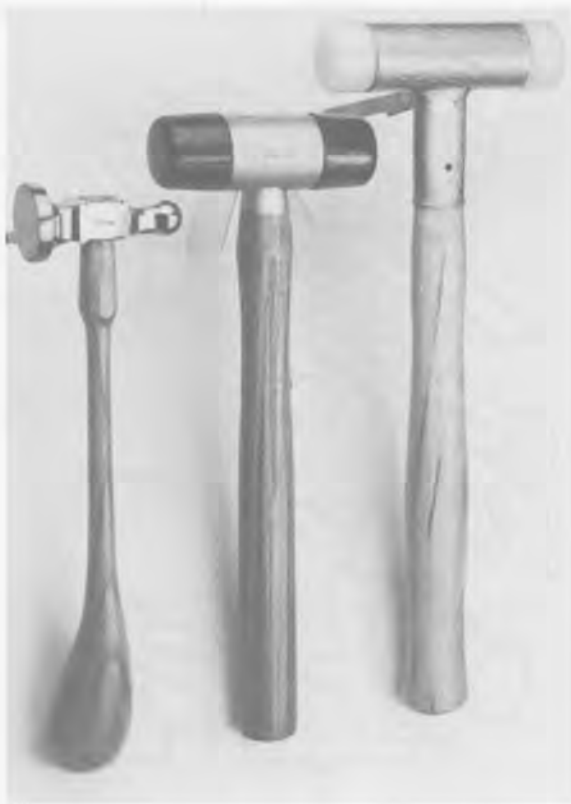
Figure 5.42 Special hammers. Chasing hammer, "Nylotex" plastic hammer with changeable hammer faces, bounceless plastic hammer. (Firma J. Schmatz, Pforzheim)
