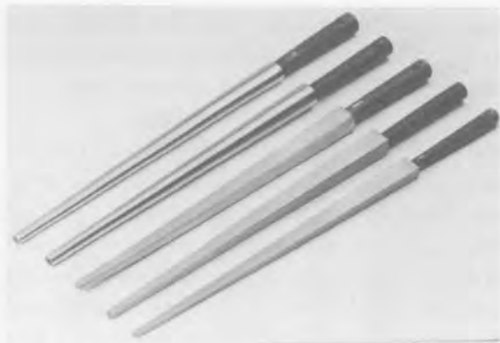
Figure 5.45 Various mandrels. Ring mandrel, angular mandrel, bracelet mandrel. (Firma J. Schmalz, Pforzheim)
