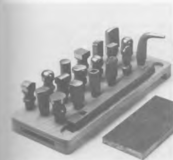
Figure 5.44 Small stake heads of different sizes with an extension arm and stake made (Firma J. Schmalz, Pforzheim)
