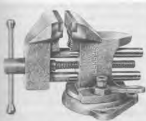
6-227 BENCH VISE WITH ANVIL Has full 360° swivel base whose position is controlled by a swivel wrench lock. Jaw width is 3 in, max. jaw opening 3 in, and has pipe-sized jaws to allow it to hold round tools such as mandrels. Weight 19 lb. Photo: Courtesy L. S. Starrett Co.
