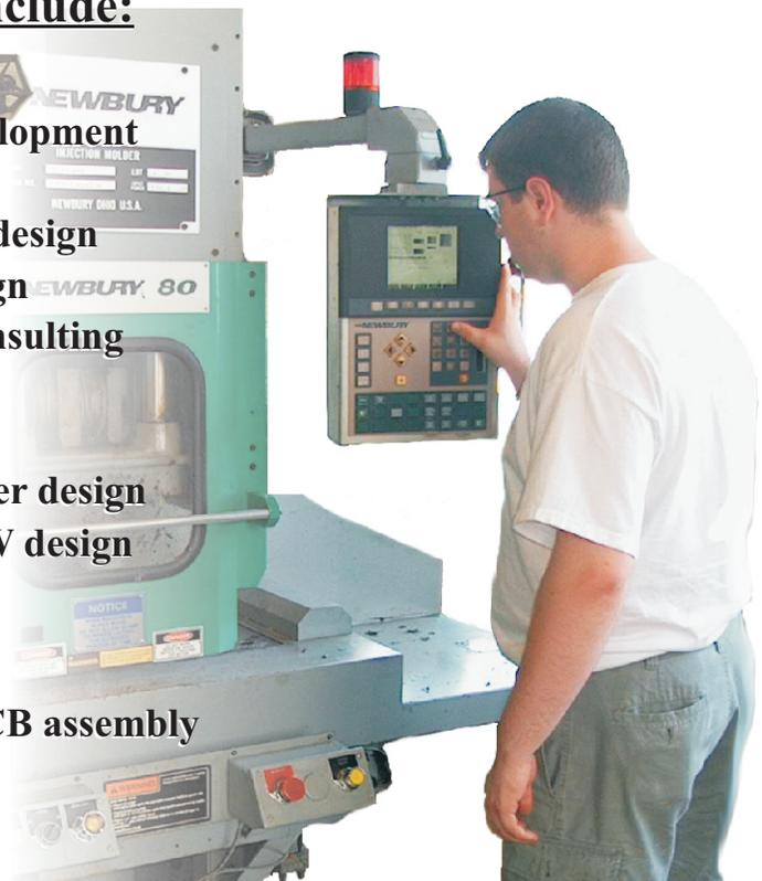
*Our 80 ton vertical injection molding machine gives us the ability to manufacture custom boots, connectors, overmolds and strain reliefs. It has the capability of injecting various types of plastic and rubber.*
