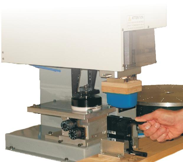
*Our pad print machine has the capability of 1,200 cycles per hour. It can also print on a variety of materials such as glass, metal, plastic and rubber.*
