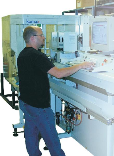
*Our wire machine has the capability to cut and crimp 4,000 pieces of wire per hour.*
