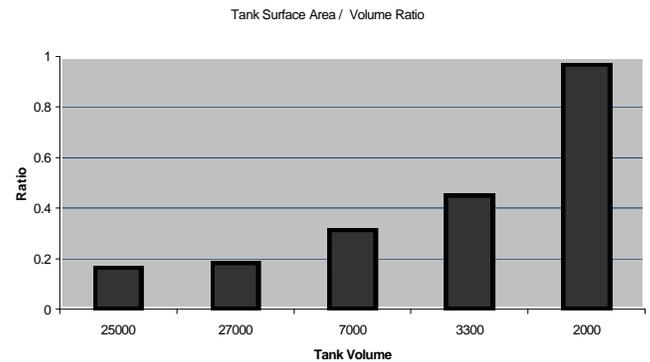
Fig. 1 Cargo Tank Surface Area vs. Tank Volume
