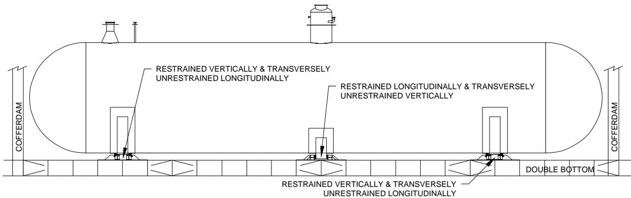
Fig 5 Cargo Tank Support and Restraint
