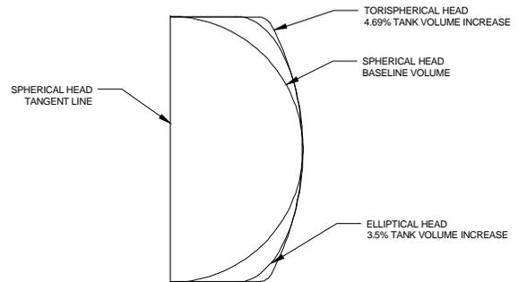
Fig. 4 Cargo Tank Head Configuration Comparison
