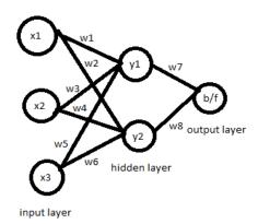
Neural networks are fully connected graphs with each node associated with an input value and each edge associated with a weight, which are initially random values and a bias added which is always set. Functioning of a neural network is carried out by calculating the weighted sum.
